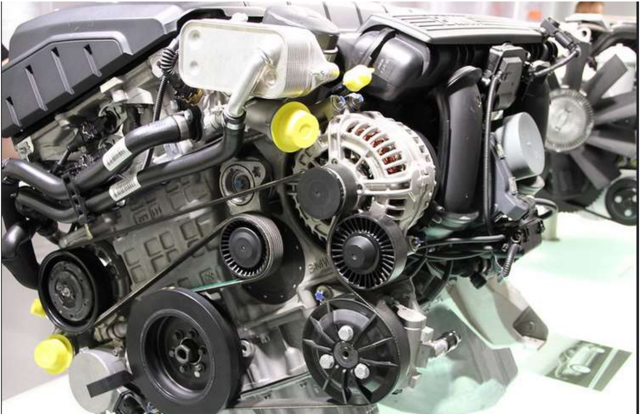
BMW 6-Zylinder-Reihenmotor, 2996 ccm, 258 PS | Foto: creativcommons/(CC BY-NC 2.0)
